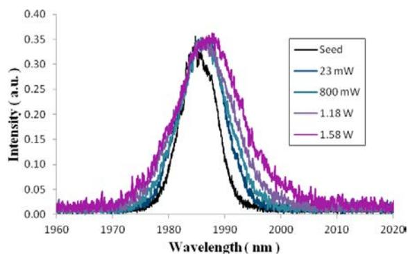
Fig. 7. Spectrum of output pulses.
