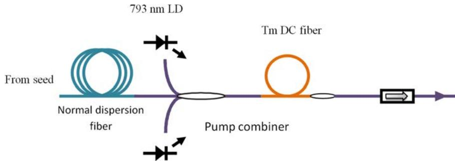
Fig. 4. First stage of amplification with pulse stretcher.
