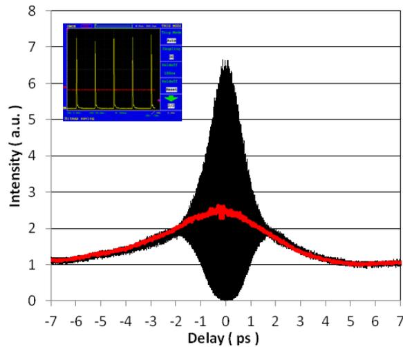
Fig. 2. Autocorrelation trace of the seed output.
