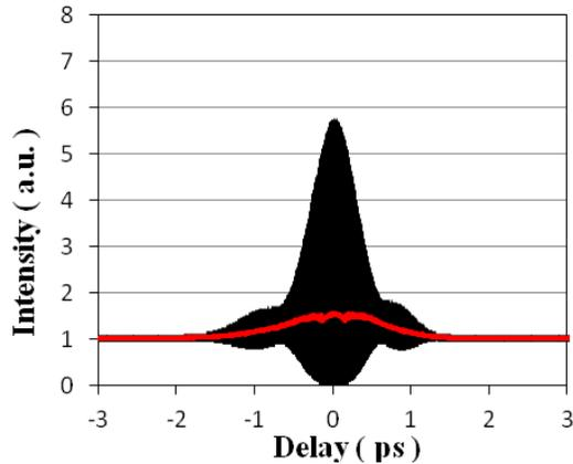
Fig. 8. Autocorrelation trace of compressed pulse.
