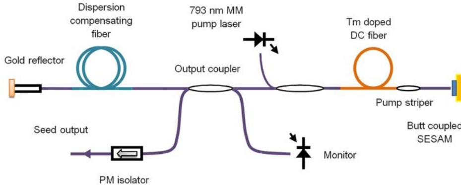
Fig. 1. Schematic diagram of the seed laser oscillator.
