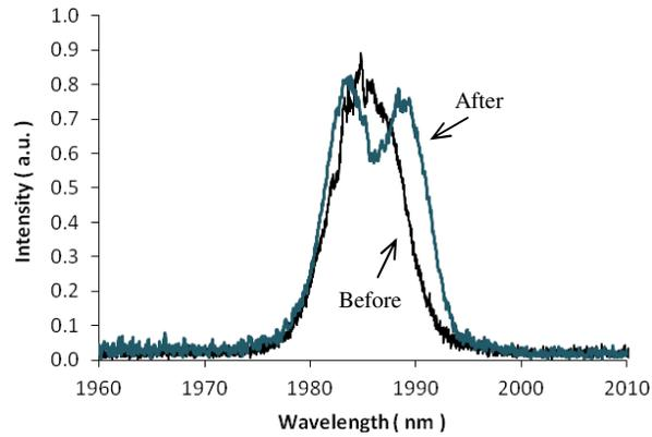
Fig. 3. Optical spectrum of seed laser before and after stretcher.
