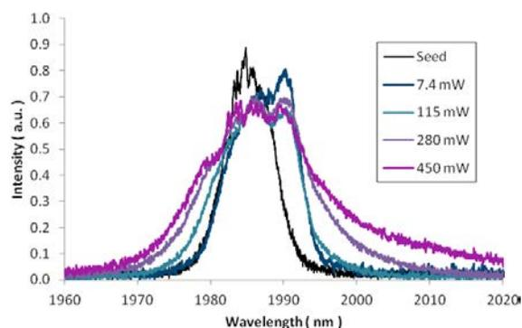
Fig. 5. Spectrum of pulses after first stage for different levels of output power.
