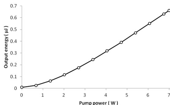
Fig. 6. Output pulse energy versus pump power of the second stage.
